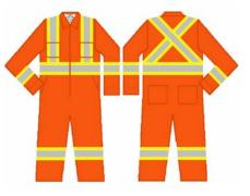
Class 3 Apparel.......Minimum areas of high-visibility material coverage requirements  $\rightarrow$  Full coverage of upper torso--- (front, back, sides, and over the shoulders), plus bands encircling both arms and both legs.
