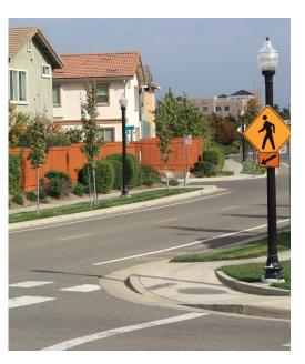
Marked crosswalks are used where vehicle volume is light (400–2,000 vehicles per hour) and the posted speed limit is under 60 kilometres per hour.
