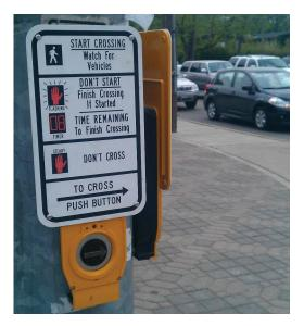
These green, amber, or red traffic lights are activated by a button on the pedestal. Once the signal is activated, vehicles must come to a full stop.
