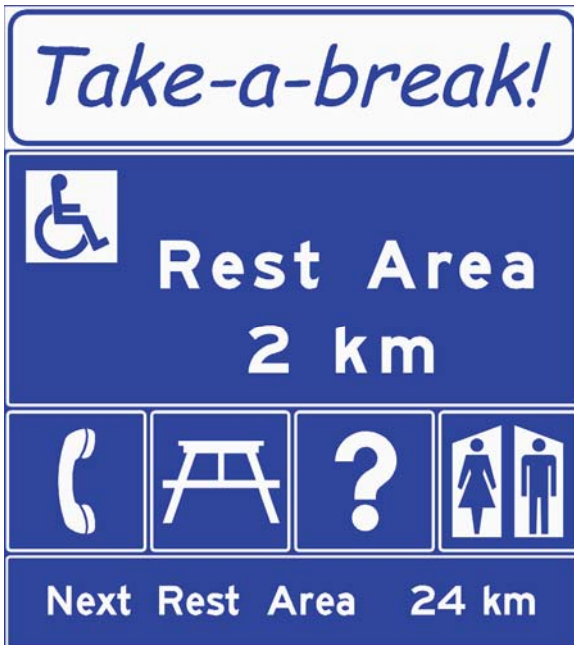
Figure 6.26 – Safety Rest Area Sign (Excludes Roadside Turnouts)
