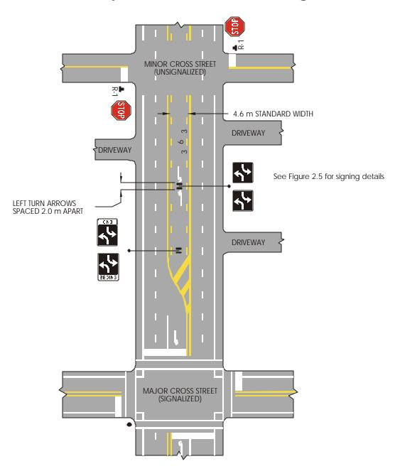
NOTE: A MINIMUM OF ONE SET OF LEFT TURN ARROWS SHALL BE PAINTED IN THE MIDDLE OF A SHORT TWO WAY LEFT TURN LANE.
