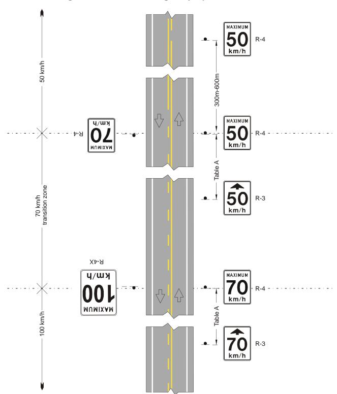
**Figure 2.1 Two-Lane Highway Speed Zone Transition**
