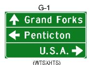
The **G-1, Destination Direction** sign series directs motorists to the next major destination or control city depending upon the geographical setting. These signs shall be erected 100m to 200m in advance of intersections and are typically shoulder mounted. In urban areas, overhead mounting may be desirable if criteria outlined in Sec. 1.9, 'General Provisions', of this manual is satisfied.
