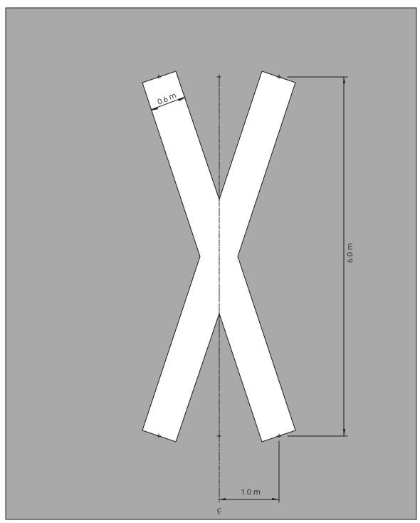
NOTE: USED IN ADVANCE OF CROSSINGS SEE FIGURE 7.42 & 7.46 FOR DETAILS PAVEMENT MARKINGS CHAPTER 7
