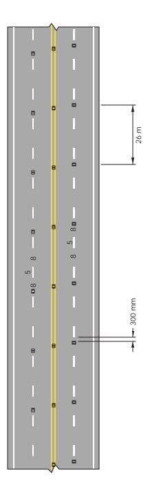
Note: Where the systematic spacing of RPMs is interrupted by a cross street, railway etc., an RPM may be moved in either direction for a distance not exceeding  $\frac{1}{4}$  of the normal spacing. If the RPM still obstructs, it should be left out and the normal spacing continued as though as RPMs were in place.
