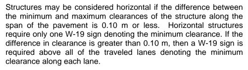
When more than one W-19 sign is installed, the W-18 LOW CLEARANCE AHEAD sign shall display the lowest clearance of any of the associated W-19 signs on the structure.
