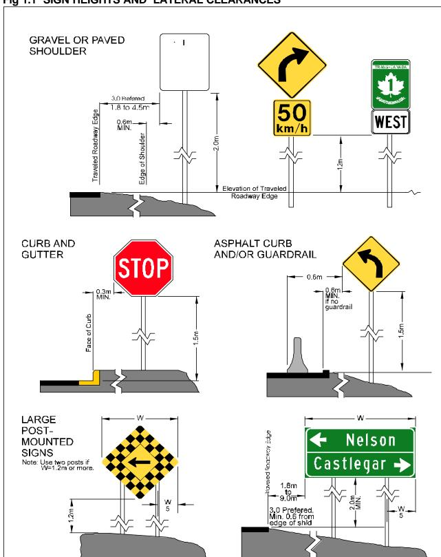
Fig 1.1 SIGN HEIGHTS AND LATERAL CLEARANCES
