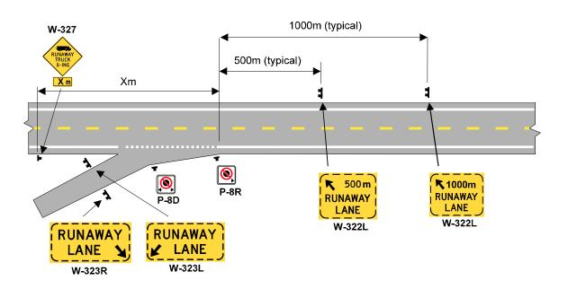
**Figure 3.3 Conventional Highway Brake Check**
