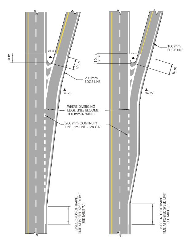
NOTE: IF THE DISTANCE BETWEEN 200 mm LINES IS < 200 m THEN CONNECT THE 200 mm LINES
