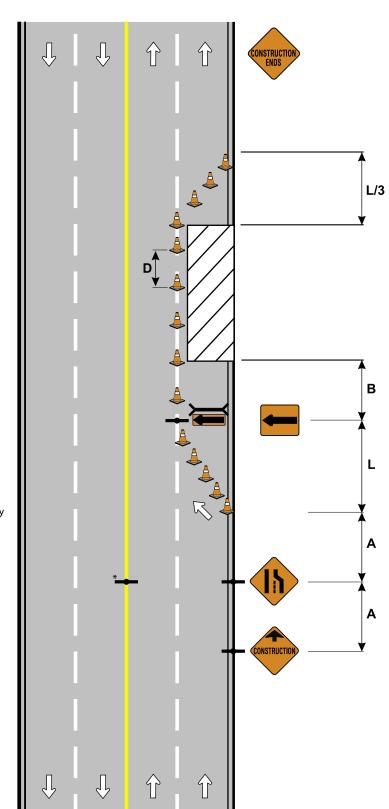
\*An additional Temporary Lane Closed Ahead sign should be placed adjacent to the left lane where median space may permit sign placement.
